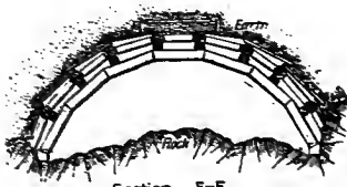
FIG. 91. — Showing Crown Bars Supported by Segmental Arches.
